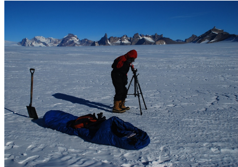
Figure 4.9: A photograph of instrumental set up (laser profilometer mounted on a tripod) at a location (71.47° S, 12.29° E) on 4 th March 2013 around Maitri station.
