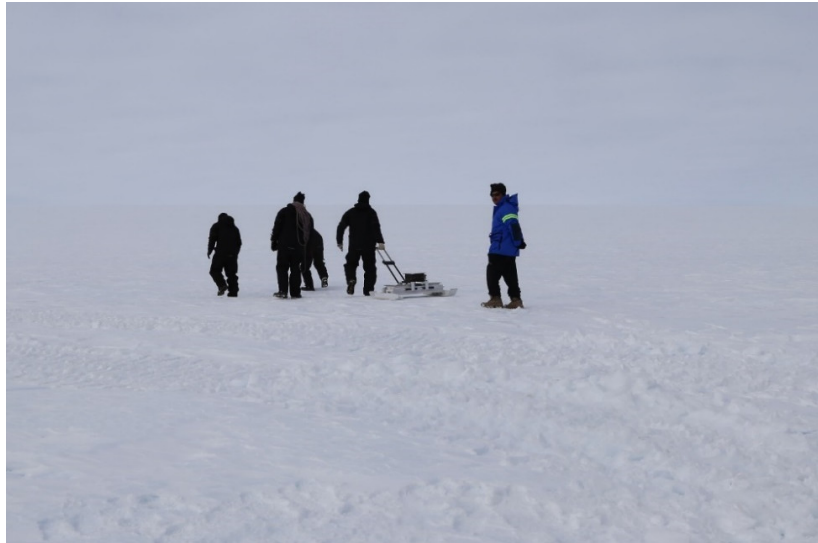
Figure 4.13: Ground observation using the ground penetrating radar (GPR) on 7 February 2015 at 69°26'S, 76°16'E.
