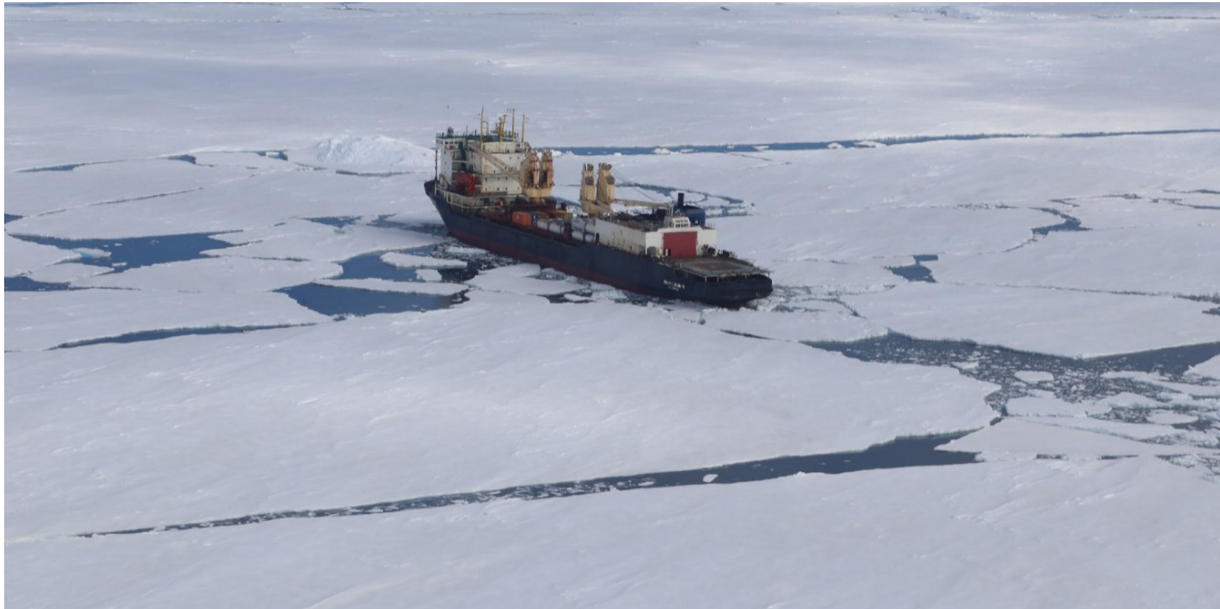
Figure 2.47: Ivan Papanin, ice class vessel surrounded by drifting large chunks of ice referred as pack ice zone. Presence of linear or straight opening in sea ice making open ocean visible referred as lead. ( 69^{\circ} 16' 44'' S, 76^{\circ} 07' 02'' E; 09 Jan 2016; 35 ISEA).
