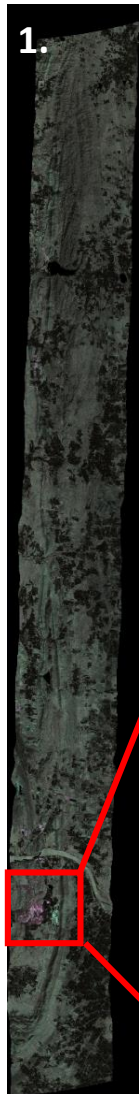
1. RGB FCC of one of the six scenes of ANG covering parts of Jahazpur region obtained by assigning 2345-nm ANG channel to Red; 2209-nm ANG channel to Green; 2389-nm channel to Blue.
