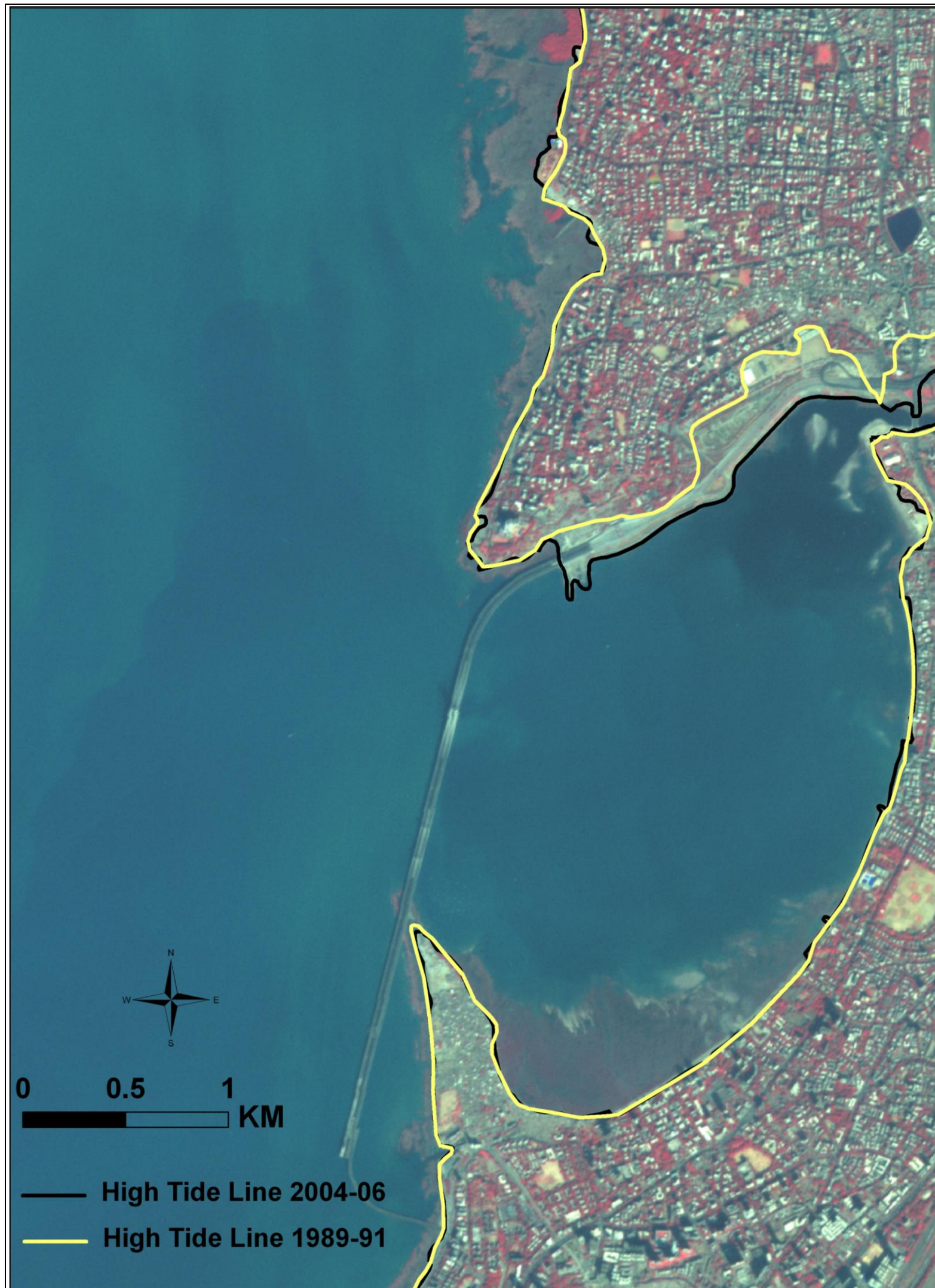
Plate 1: 2011-12 LISS IV image overlaid with high tide line of 2004-06 and 1989-91, showing reclamation of land for constructional activities near Mahim Bay in Mumbai (47A16SW).
