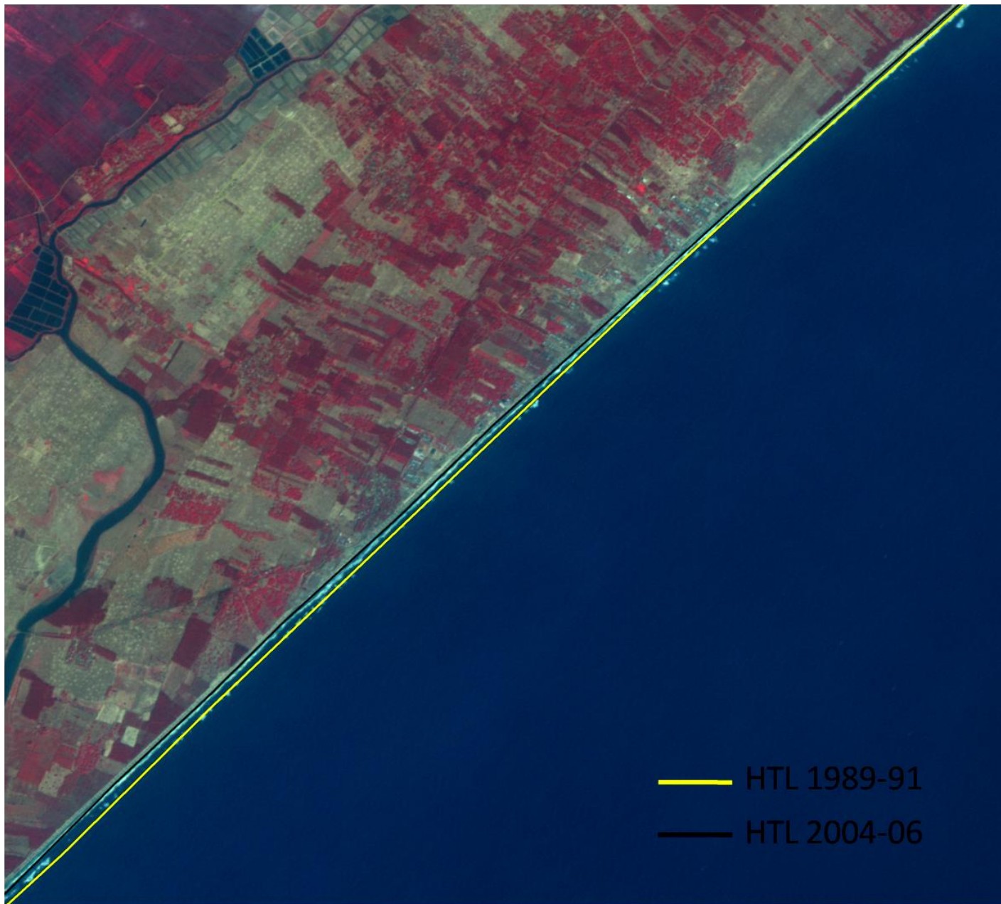
Plate 7: Severe erosion from Avulamanda to Shamvanipakalu coastal stretch in East Godavari district (65K08NE, 65K08SE)
