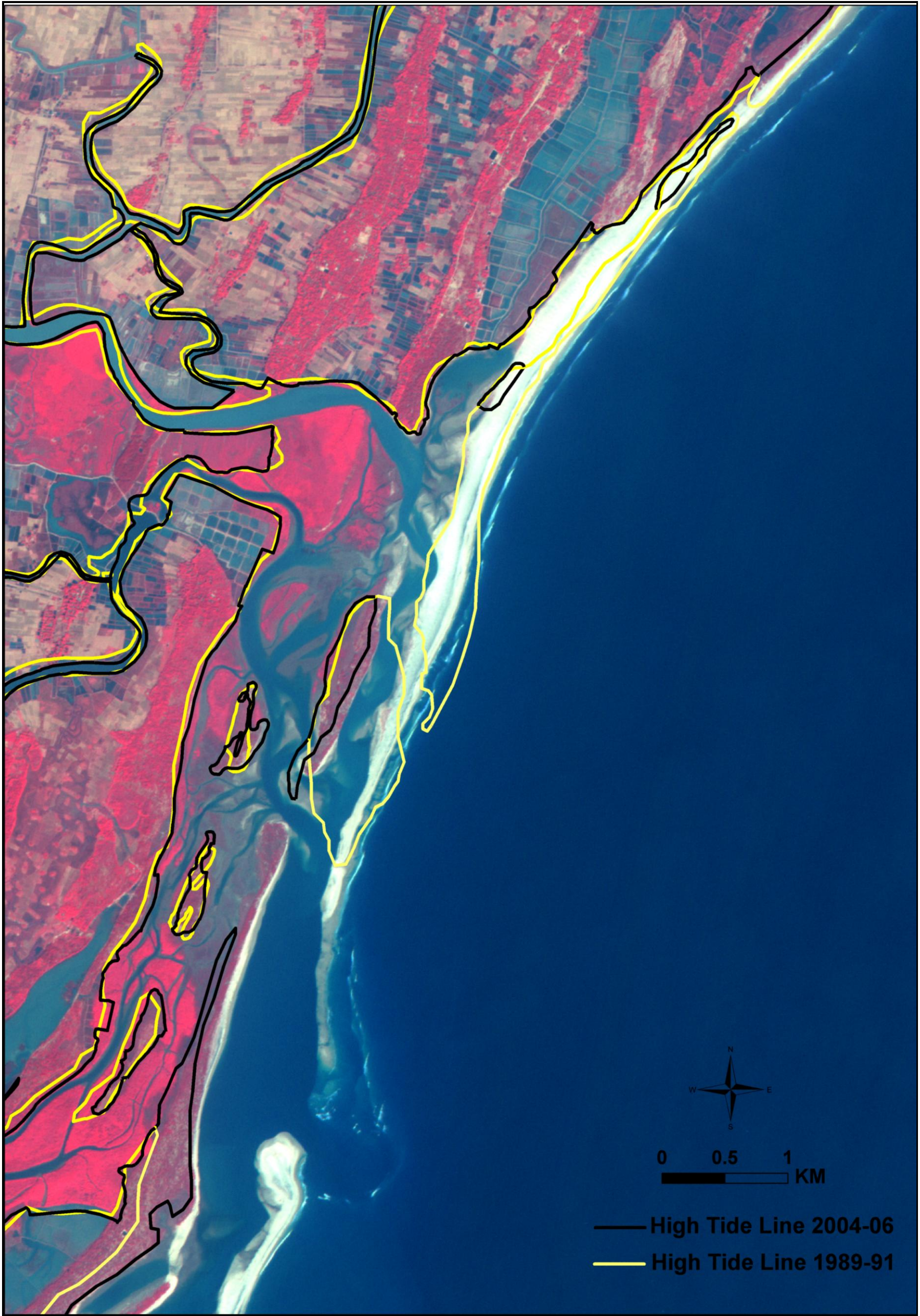
Plate 3: 2011-12 LISS IV image overlaid with high tide line of 2004-06 and 1989-91, showing severe erosion at Bhitikolia River mouth (73L08SE).
